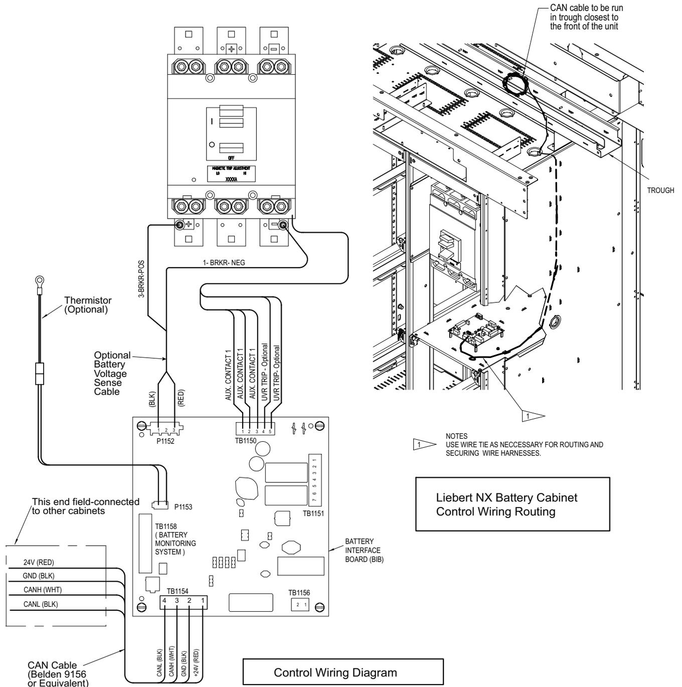
Figure 17 Attached battery cabinet connections
