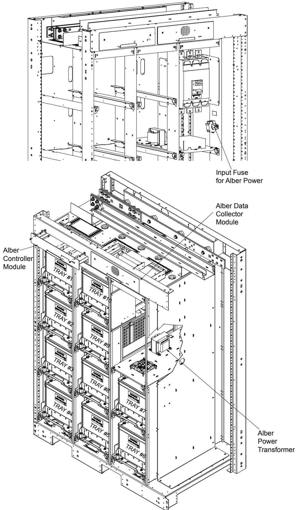
Figure 20 Alber battery monitoring wiring to multiple battery cabinets
