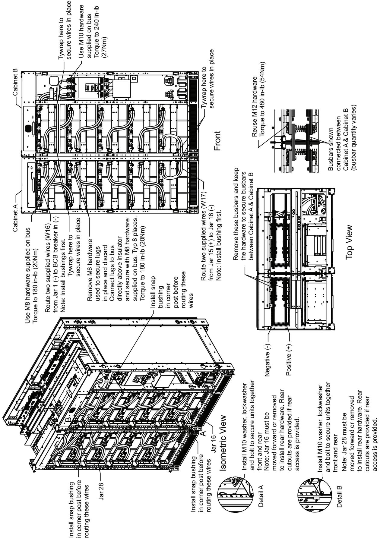
Figure 12 Front Terminal Battery Cabinet main components, layout
