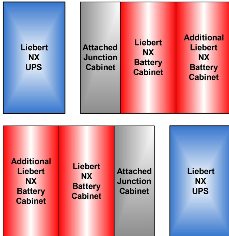
Figure 4 Stand-alone battery cabinets, detached from UPS
