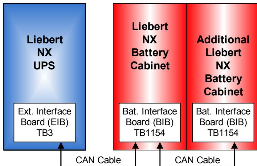
The CAN cables must be two, twisted pair, shielded 18AWG (Belden 9156 or equivalent). All interconnecting cables and hardware for connected and attached cabinets will be provided.
