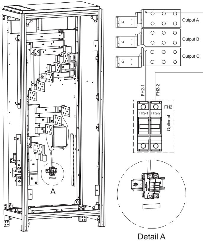
This harness is intended for use only when battery cabinet is connected directly to UPS. For all other instances, customer must supply wire. Secure supplied wire harness to busbar with supplied hardware.
