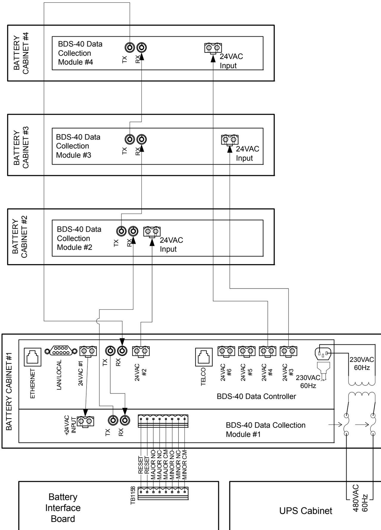
Figure 21 Alber battery monitoring assembly diagram
