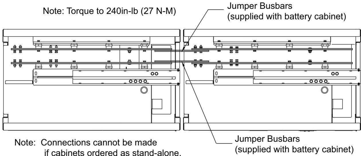
Figure 18 Ground strap location for connected cabinets
