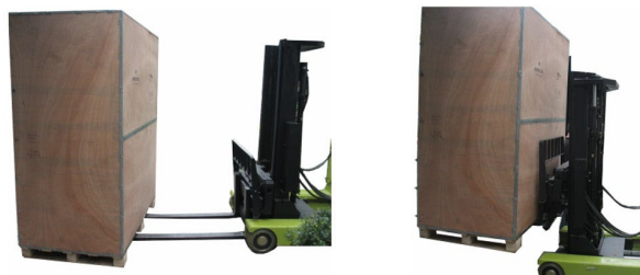
Figure 2-1 Inserting and movement
