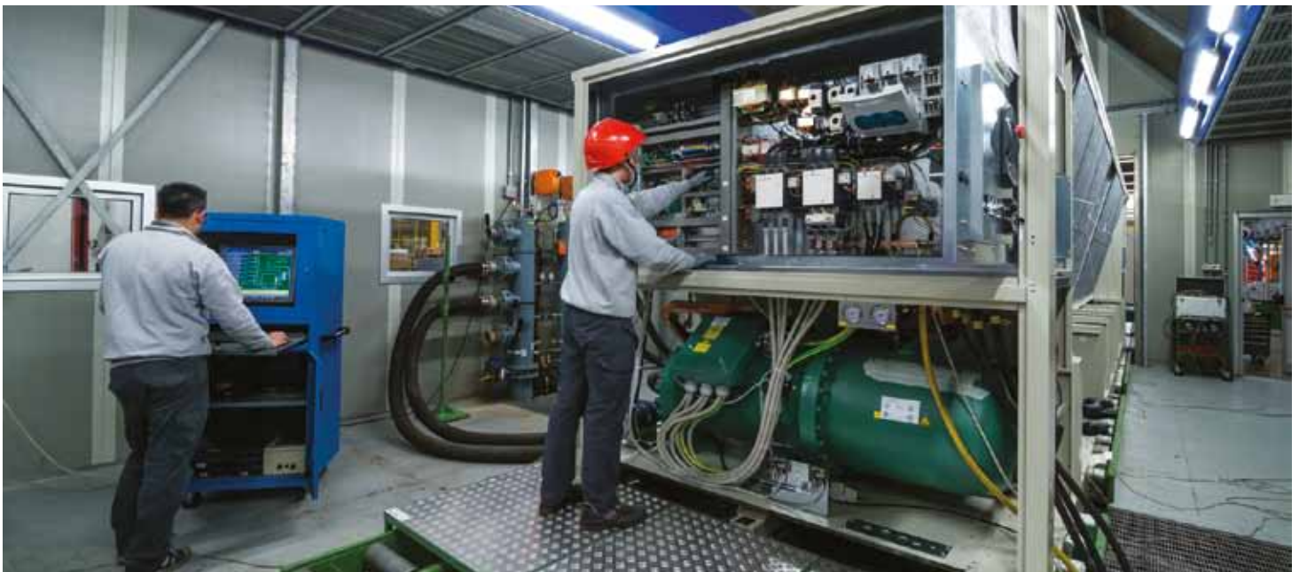
Witness test cabins have been designed to optimize the reliability of unit testing, ensuring that real installation conditions are simulated in order to confirm the unit's guaranteed performance.
