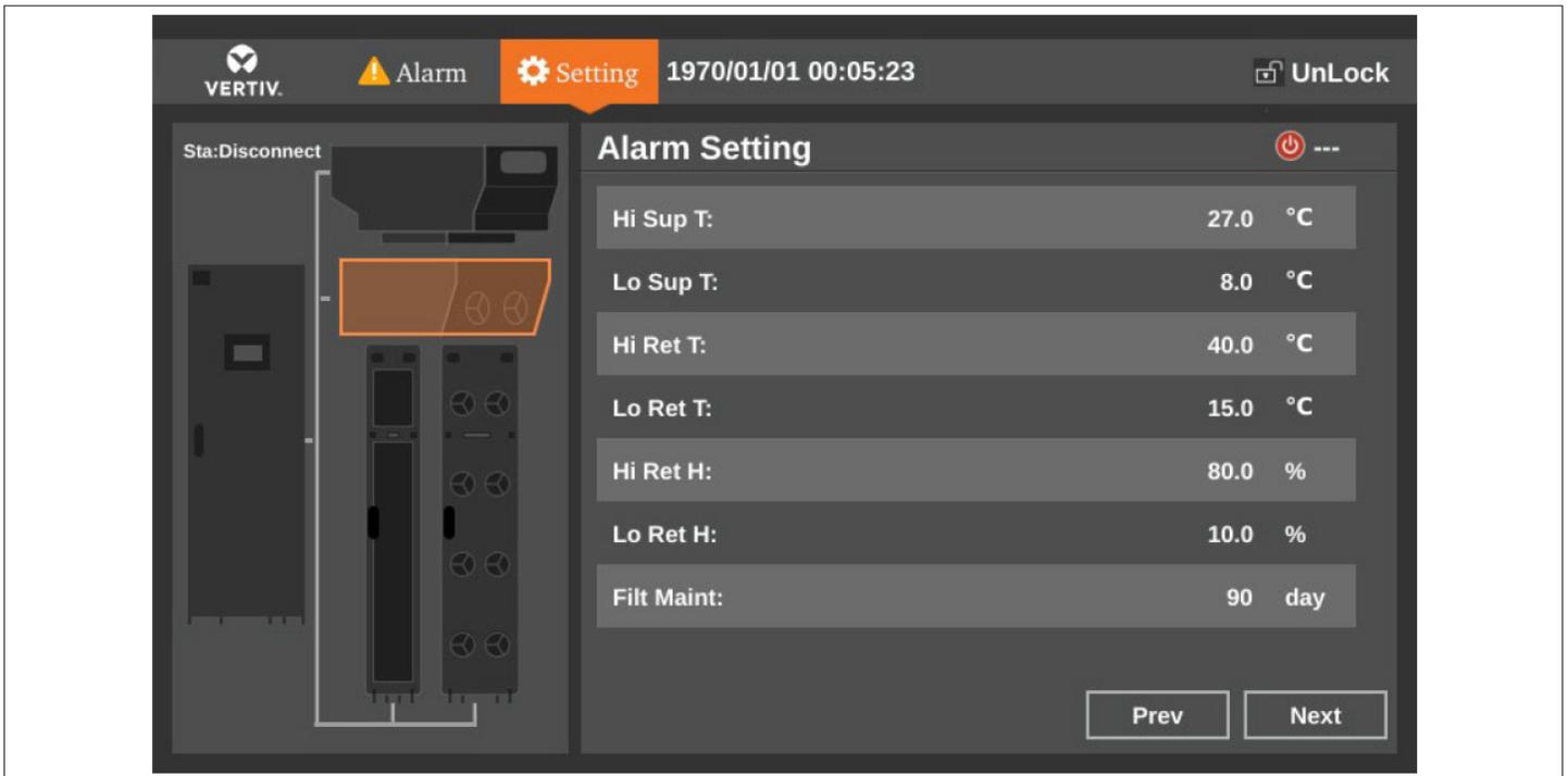
**Figure 5-11 Terminal Alarm Setting Interface**
