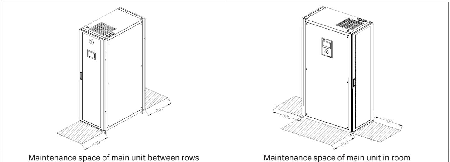
**Figure 2-1 Schematic Diagram of Unit Maintenance Space**
