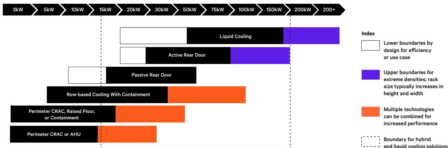
Liquid-cooled systems are often used with air-cooling systems to cool racks at higher densities.
