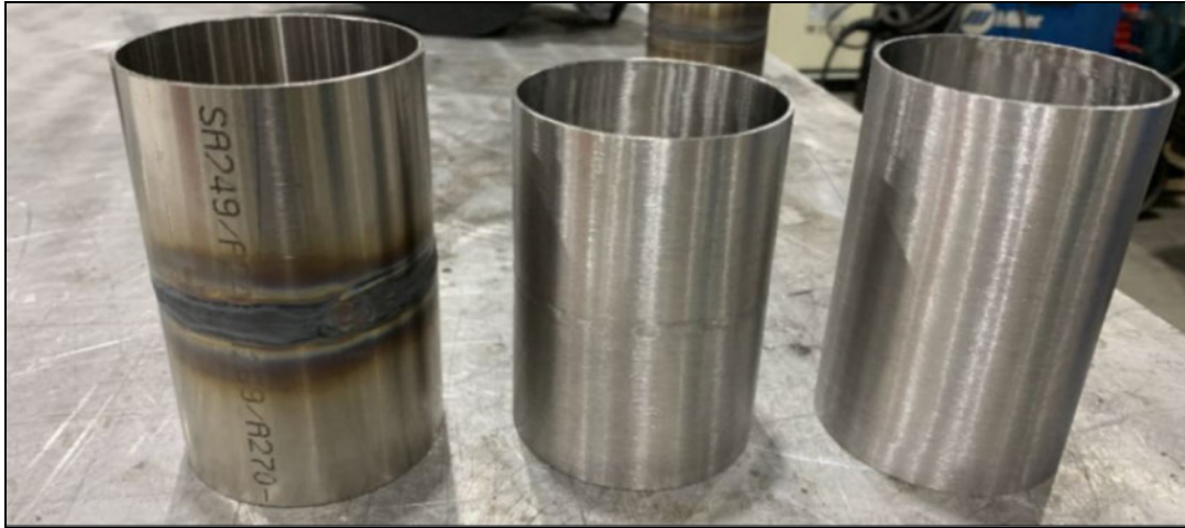
Figure 5.2 Treatment Levels of Welded Joints
