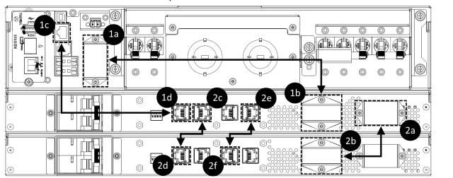
GXT5 Lithium-Ion UPS to External Battery Cabinet Connections
