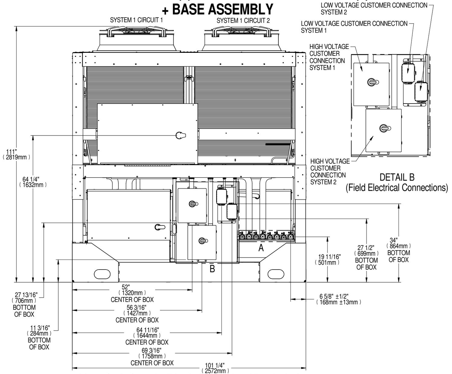
ALL CONNECTIONS MADE FROM SYSTEM 1 END OF UNIT (SHOWN)
