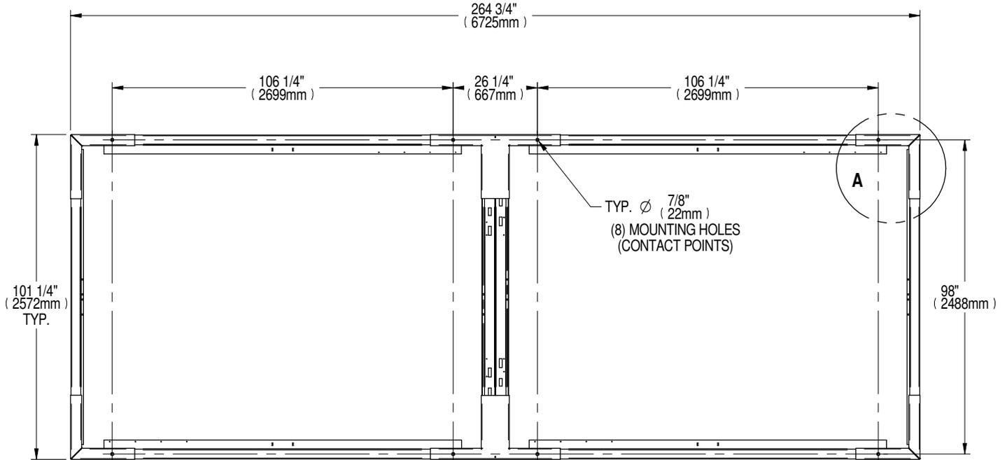
Underside of unit, coil and fan removed for clarity.
