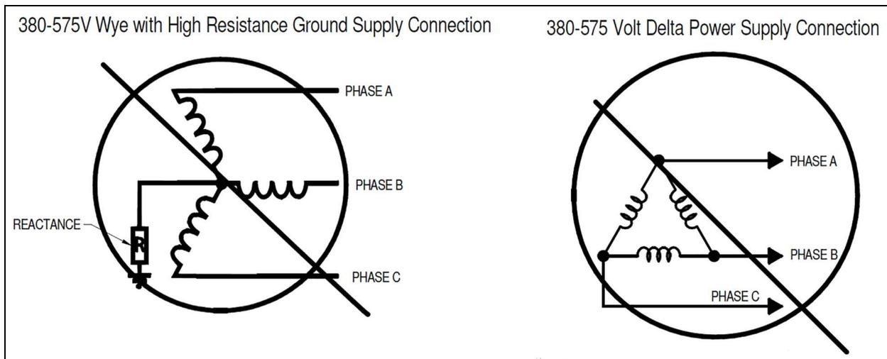
**NOTE:** The 380-575 volt unit is designed to operate with Wye-connected power with a solidly grounded neutral. It will not operate properly with Wye-connected power with high-resistance (or impedance) ground or with Delta-connected power. A separate neutral wire is not required to be run to the Liebert® MCV Condenser.
