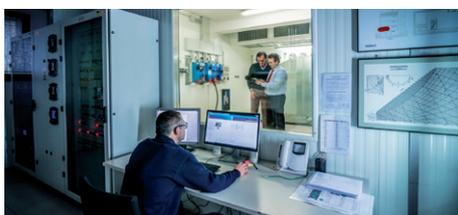
The Research & Development Validation Lab 1 is specifically designed to test floor-mount units and can balance a thermal load of up to 150 kW with a chamber air temperature between 0°C and 60°C.
