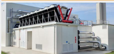
This latest designed lab can test units with cooling capacities up to 1.5 MW with state-of-the-art accuracy in a broad range of working conditions, from -10°C to +55°C, also for adiabatic units.
