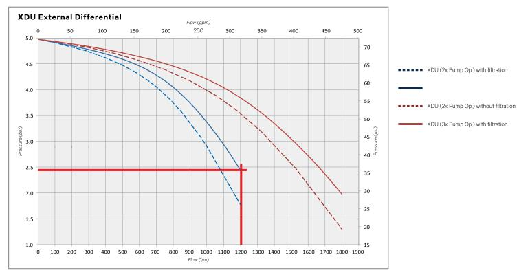
317 gpm (1200 l/m) at 35.4 psi (2.44 bar) differential pressure external to
