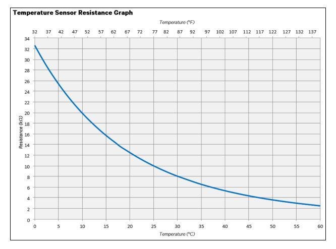
This chart may be used to check the validity of the 10 K thermistor temperature sensors used in the unit.
