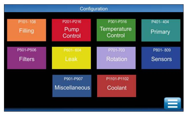
NOTE: Parameter IDs shown in red text will only be accessible with the Engineer log-in code.
