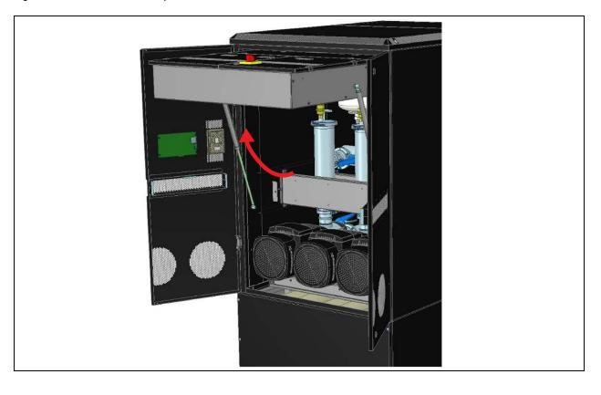
Figure 5.1 Access to Secondary Filters with Electrical Panel in Horizontal Position
