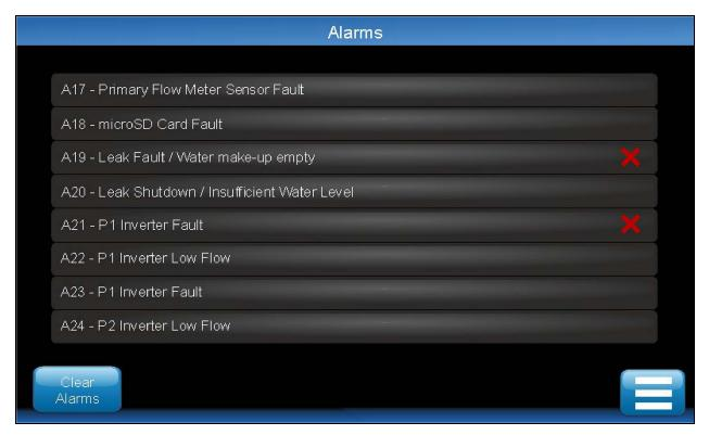
Some alarms will 'self-clear' if the condition is a brief one (e.g. a temperature goes over an alarm threshold then comes back to a healthy condition) or when the fault has been rectified (e.g. a faulty sensor has been replaced.)
