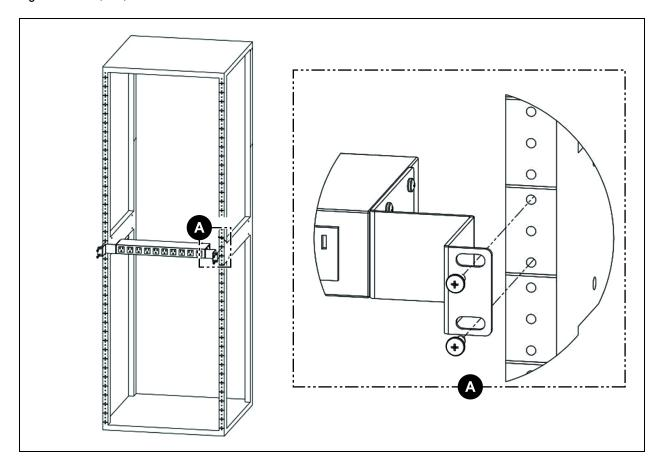
Figure 3.13 19" (inch) Horizontal/Panel-Mount Brackets
