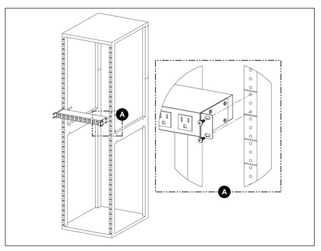
Figure 3.10 Adjustable Mount Bracket
