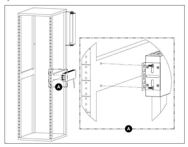
Figure 3.12 23" (inch) Conversion Mount Brackets
