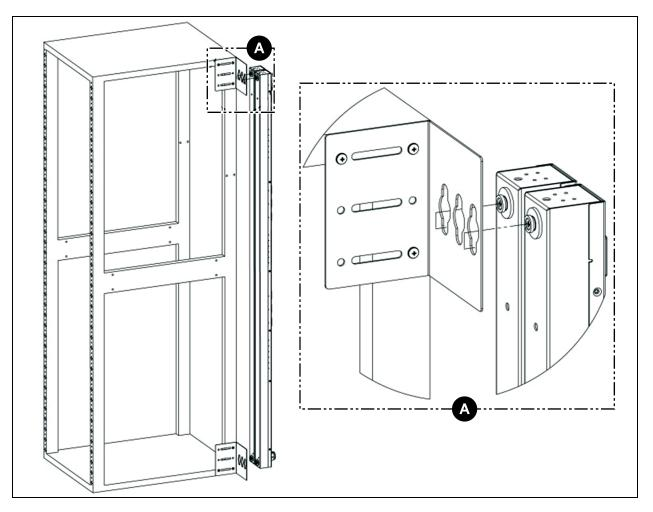
Figure 3.7 Offset/Side Mount Brackets
