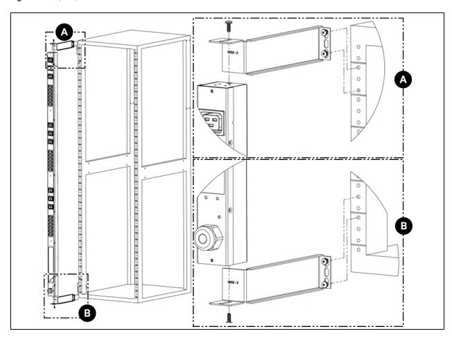
Figure 3.9 Flush Mount Bracket
