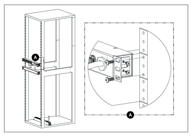
Figure 3.14 Mount Brackets for Vertiv™ PowerIT Universal Power Distribution Unit (UPDU) with Pivoting End
