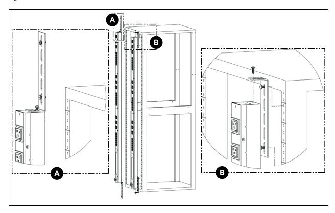
Figure 3.4 Toolless Mounting Hardware
