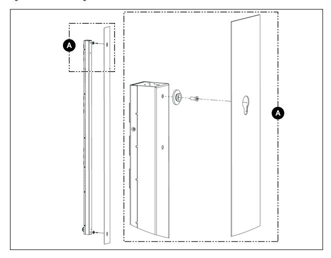
Figure 3.5 Toolless Full Length Brackets
