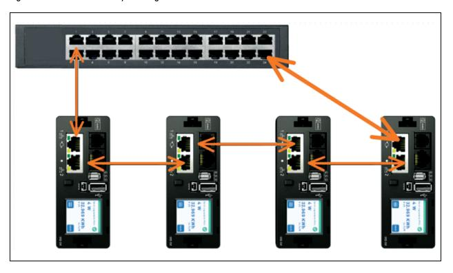
When both network interfaces are connected, the IMD implements a network bridging protocol called the Rapid Spanning Tree Protocol (RSTP). RSTP is an IEEE standard that is implemented by all managed bridges. Using RSTP, bridges in the network exchange information to find redundant paths or loops. IPv6 should be disabled when using redundant network connectivity.
