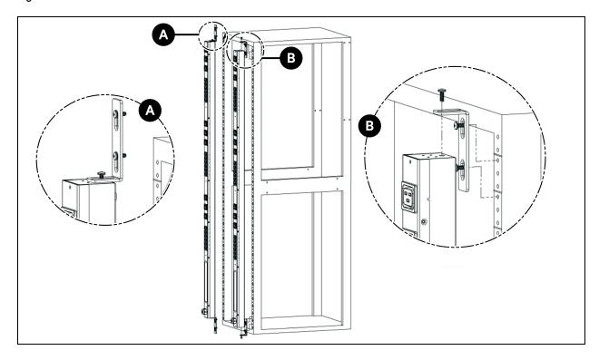
Figure 3.3 Vertical Extension Brackets
