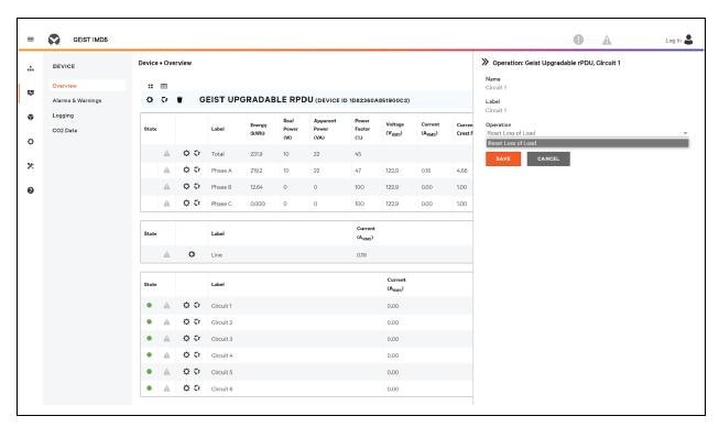
NOTE: This step is required when state shows a loss of load alarm and the issue has been resolved. Loss of load alarm is triggered by a sudden drop of current detected by the circuit breaker's current measuring transducer when operating close to the circuit load limit. For the Switched Upgradeable horizontal units, the loss of load alarm is additionally triggered by circuit breaker loss of voltage (regardless of circuit load).
