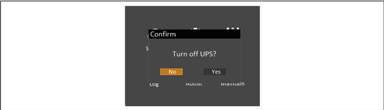
In Inverter mode, press and hold the power button. If the bypass is abnormal, then the interface shown in **Figure 5.9** below is displayed, select 'YES' to shut down the UPS output.
