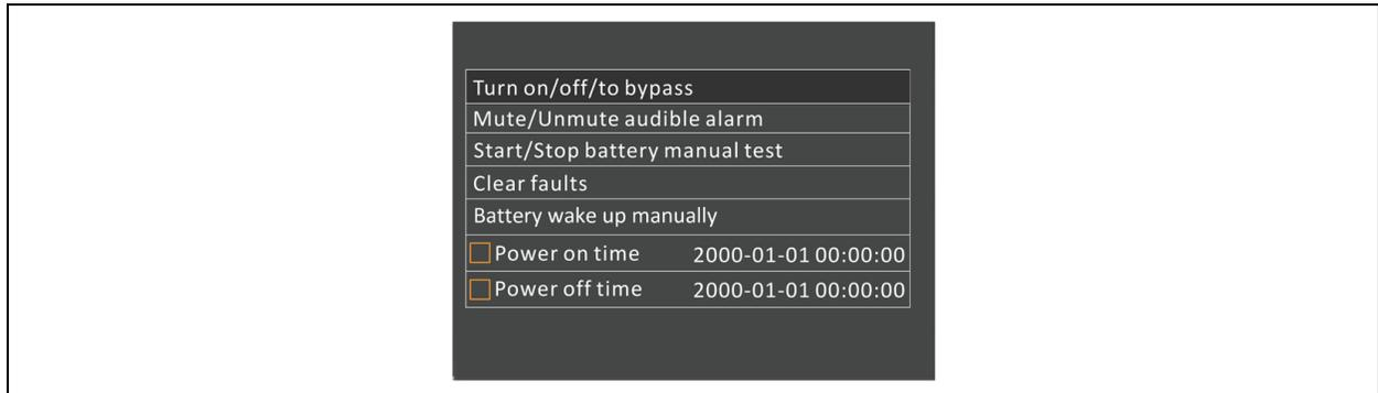
The Control page contains the Turn ON/OFF/to BYPASS, and Manual battery test. Refer to the in **Figure 6.24** above.
