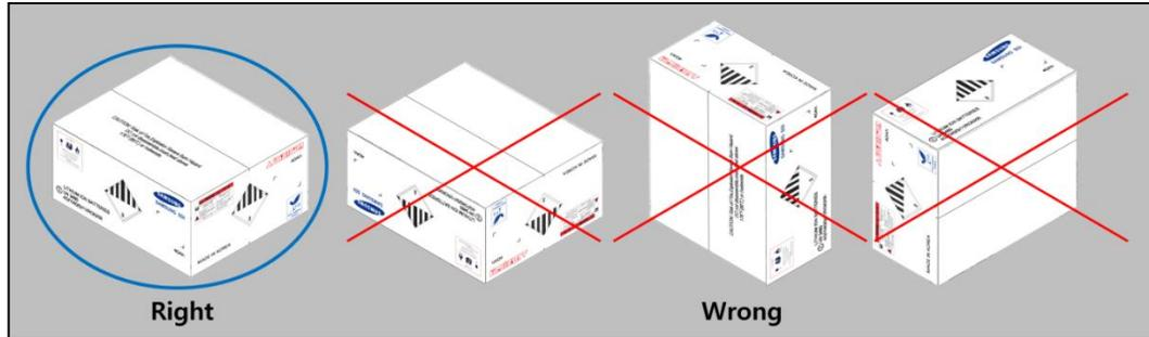
[Fig 1] Module Storage Method
