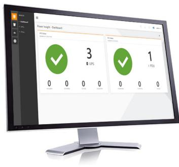
**Vertiv™ Power Insight** is a web-based solution for managing and monitoring up to 100 Vertiv™ UPSs and Vertiv™ rPDUs that provides a quick way to safely shutdown IT devices based on user-configured parameters.
