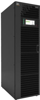
The row-based Liebert® EXM is a transformer-free, on-line UPS that provides modular hardware scalability and N+1 redundancy from 10-200kVA in 208 volt configurations and 50-250kVA in 480 volt configurations.
