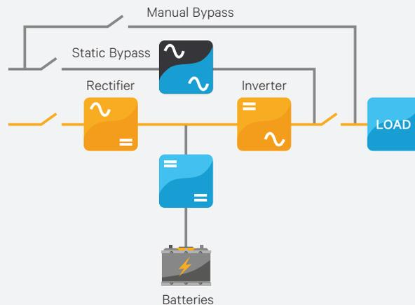
**Intelligent ECO Mode (VFD)** detects when conditioning is not required and allows the energy flow to pass through the bypass line.
